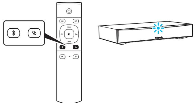
3. Consult the instructions of the Bluetooth device to connect to TV2. Successful pairing will be signalled by a 'beep' from the unit and the Blue LED
