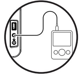
Press the **AUX** button to select the Aux input. There is an Aux input on the rear of the unit that allows any analogue device to be connected. LED will turn green to indicate Aux input is selected.
